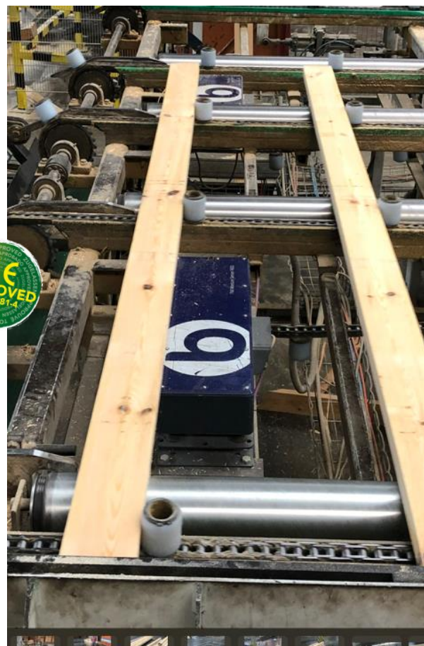
FMI sensor transversal wood transport
