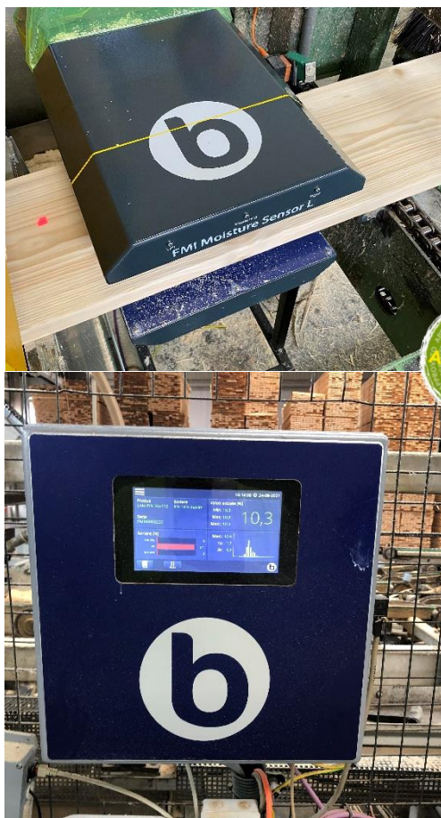
FMI Sensor longitudinal wood transport FMI Operating Panel
